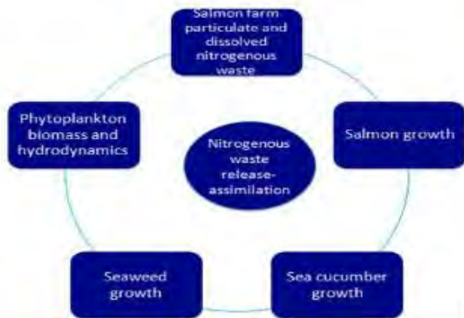
Figure 1: IMTA model outline. The model consists of five sub-models interconnected via relationships of nitrogen release and assimilation.
